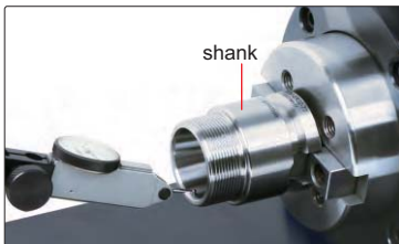
measure radial runout of shank
