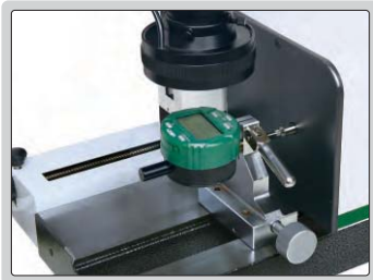
check digital indicators (detect digits on screen)
