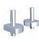
Measuring external groove diameter with flat measuring face (depth h1 \leq 2.5mm )
