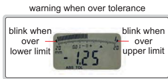
warning when over tolerance
